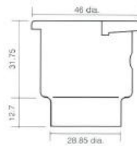
NECK 04422000AAB (PRESSING) material 0.91 thick mild steel
